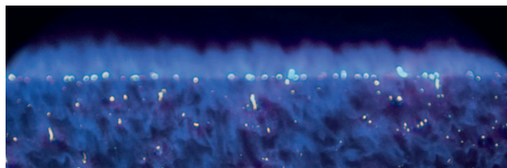
The homogeneous mixture of gas and air combusts on the surface of the woven metal mesh at temperatures < 1200 °C. This combustion technology effectively inhibits the formation of thermal NO x .
